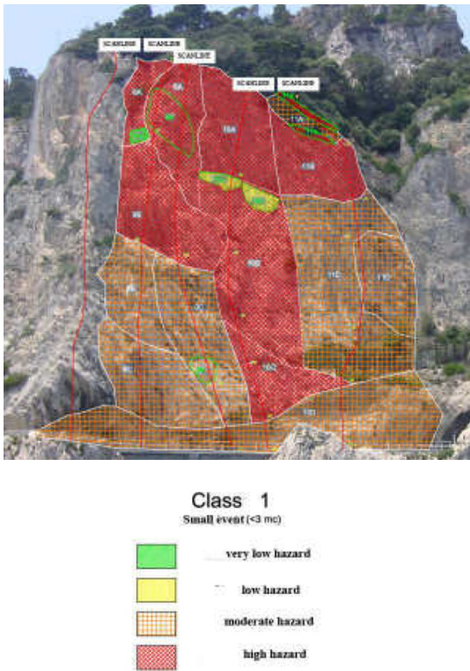
Fig. 5 –Landslide hazard zonation with respect class 1 events.
